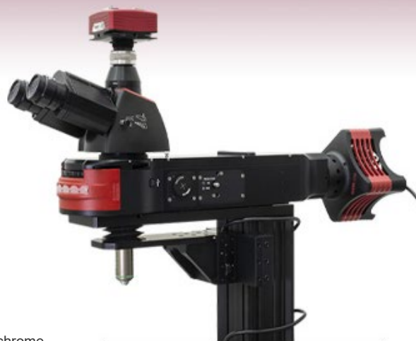
Scientific CCD Camera in a Cerna ® Microscope
